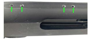
Begin by removing the (4) existing set screws from the top of the receiver using a flat head screwdriver as seen in (Flgure 1a)
