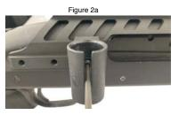
Place the add-a-shell onto the side saddle and using the provided 10-32 x 3/8" button head screw (#1) and the lock washer (#4), tighten the add-a-shell to the side saddle using a 1/8" allen wrench as seen in (Figure 2a). You may mount up to 6 add-a-shells to the non-ejection port side and up to 3 on the ejection port side.
