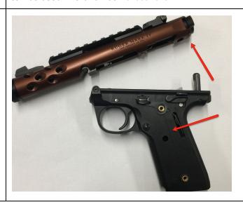
3. Uncock the pistol. Place an unloaded magazine into the pistol, put the pistol on fire and pull the trigger. Alternatively you can lift the magazine safety with a tool and pull the trigger.
