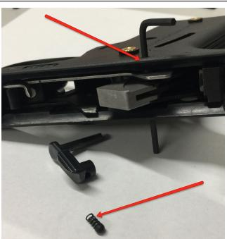
5. Install the Ruger factory provided spacer over the shaft on the "Cornerstone" and reinstall the factory screw into the end. This will keep the "Cornerstone" in place and allow it to properly function. Do not overtighten. The "Cornerstone" should move freely up and down with the detent clicking it into place.
