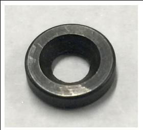
The spacer is .080" thick and has a recessed face for the tapered screw found in the safety. As a replacement an aluminum spacer from McMaster-Carr with a drilled surface can be used. Part number: 94669A029
