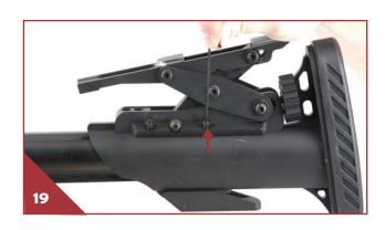
After you have the tension of the slide adjustment of the stock set, tighten the 2 nuts on each side of the stockbody using a 3/8" open face wrench, to insure the tension is locked in place as seen in Figure 20. Apply 10 ft/lbs. of torque to the nuts to ensure they do not come loose.
