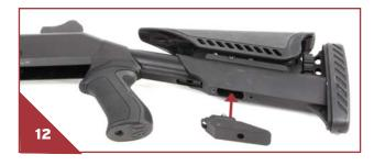
Using (2) 8/32 x 1/4" button cap screws and a 3/32" allen wrench tighten the buttstock LOP lever to the bottom of the stock body.
