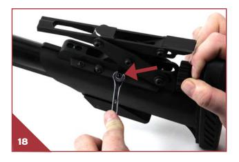
Next, use a 3/32"" allen wrench to loosen or tighten the (2) set screws on each side of the stockbody as seen in Figure 19. By loosening or tightening these set screws you will be able to set the tension of the stock on the buffer tube. Adjust all (4) set screws in small increments, testing the tension in between each adjustment of the (4) set screws until the desired tension is achived to insure that the stock slides uniformally on the buffer tube.
