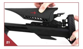
Use a T20 torx driver and tighten the screw in the front of the cheekrest to secure the cheekrest to the stockbody as seen in Figure 22.
