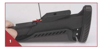
After unscrewing the LOP lever, pull down and remove the latch from the buttstock as seen in Figure 2.
